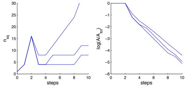
Figure 6. To illustrate the convergence of the algorithm, 100 random examples with 3 cameras and 20 points were constructed. The plots show the median and the first and ninth decile of the data. In the left plot the number of squares left after each step is shown and the right plot shows how much of the total area these squares constitutes.
