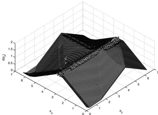
Figure 4. In the figure is shown the function  $d_z(\theta)$  as a function of  $(\theta_2, \theta_3)$ -parameter space while keeping  $\theta_1$  fixed, for the data in the example with 3 views of seven points. Notice that the function is periodic so for this particular example there is only one local minimum.
