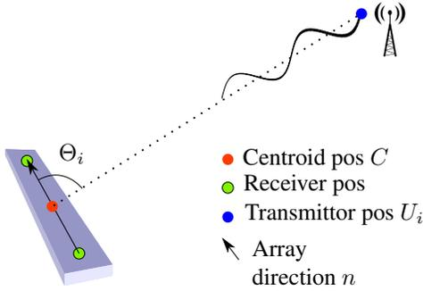
**Figure 1.** Two receivers with centroid  $C$  and direction  $n$  measuring angles  $\Theta_i$  from transmitters  $U_i$ .
