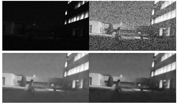
Figure 2. Upper left: One frame of the original sequence. Upper right: Tone mapped version. Lower right: After noise reduction. Lower left: After intensity stretching.
